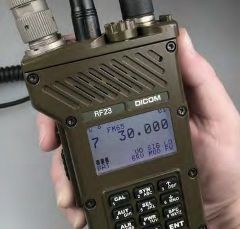
The RF23 handheld multiband transceiver designed for squad, team, platoon, and company operations, features superior resistance against radio-electronic warfare.
