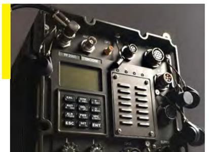
The RF2350 multiband mobile transceiver designed for installation in all tracked and wheeled vehicles and base stations, features superior resistance against radio-electronic warfare.
