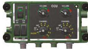
Two (ANR) headsets with full access to the intercom; CNRs can also be connected to the CCU. The unit is designed to connect two senior crew members with two top-priority, galvanically isolated CNRs.
