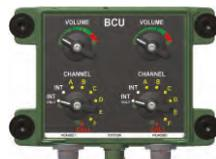
Two (ANR) headsets can be connected to this unit, providing full access to the intercom and CNRs, with independent volume control for crew members.
