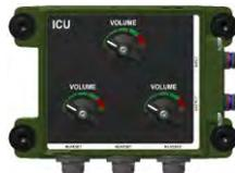
Three (ANR) crew members can be connected to the ICU with access to the intercom. Crew members connected to the ICU can also monitor CNRs.
