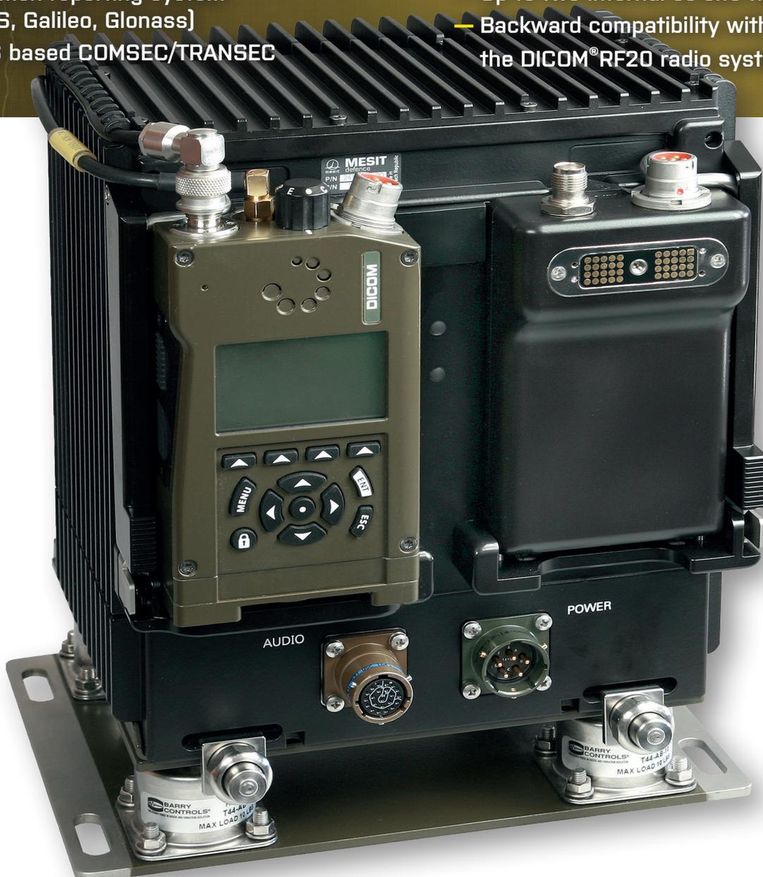
The RF4050 multiband, multirole VHF/UHF vehicular radio is designed for communication on the tactical level in all military branches.
