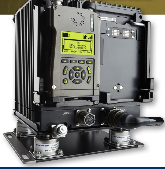
The RF4050 multiband, multirole VHF/UHF vehicular radio is designed for communication on the tactical level of command of all services.
