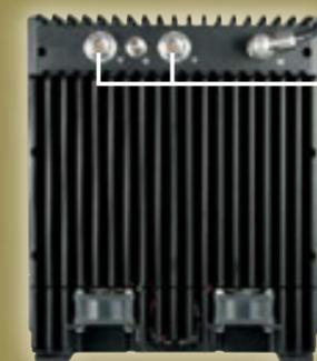
The RF4050 vehicular radio consists of the RF40 handheld radio and an amplifier block into which the radio is docked. Docking of the radio provides its firm mechanical attachment and system interconnection through a multi-pin nut connector and power connector on the back of the radio.
