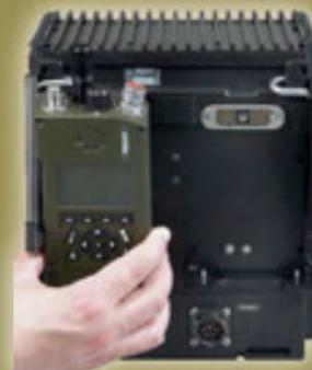
Docking of the radio into the amplifier is controlled by only one element, allowing for a very easy and fast removal of the radio - Jerk&Run support.
