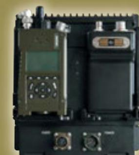
The RF4050 multiband, multirole VHF/UHF vehicular radio is designed for communication on the tactical level in all military branches.
