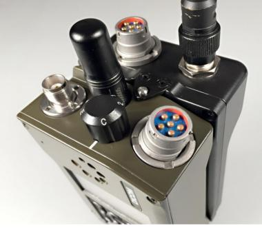
The RF40V multiband, multirole VHF/UHF vehicular radio is designed for communication on the tactical level in all military branches.
