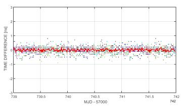
Example of a short baseline comparison error, CGGTTS V2E data, GPS L1 C/A signal, 31 satellites.
