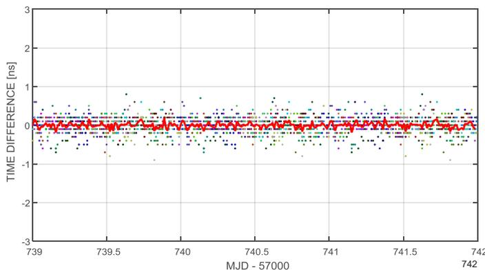
Example of a short baseline comparison error, CGGTTS V2E data, GPS L1 C/A signal, 31 satellites.
